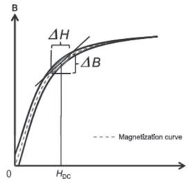
If the amplitude of the alternating field  $\Delta H$  is negligibly small, the permeability is then called **reversible permeability**,  $\mu_{rev}$ . Once the bias  $H_{DC}$  approximates to 0, the reversible permeability will revert to initial permeability. The behavior of the reversible permeability is normally shown in the characteristic curves with the subject of 'Permeability v.s. DC Bias field' for the metal dust cores featuring distributed gap.
